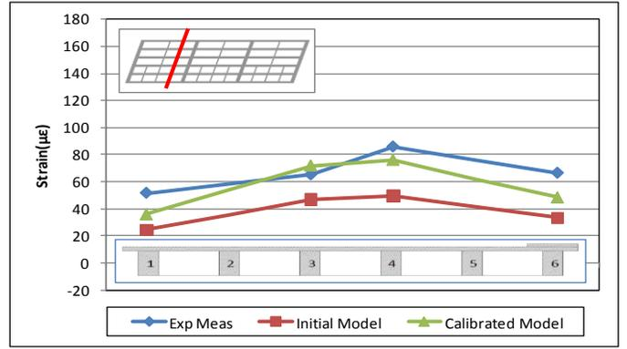
Figure 6. Comparison of the strain before and after the elastic modulus updating for 1/4, 1/2 and 3/4 line.
