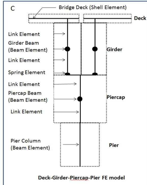
Figure 3. Finite element model and the detailed configuration.
