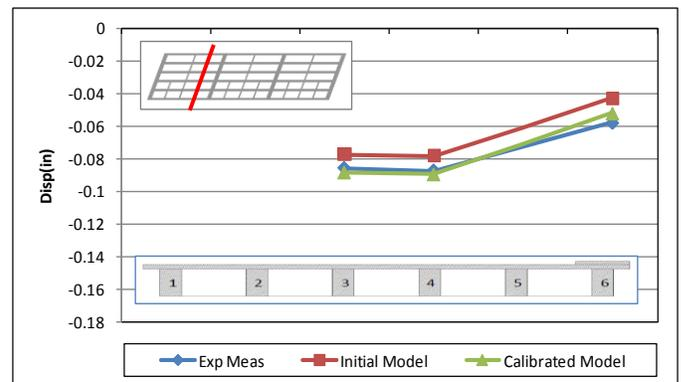
Figure 9. Comparison of displacements before and after average crack height  $y$  updating for 1/4, 1/2 and 3/4 line.
