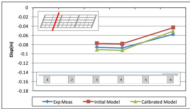
Figure 5. Comparison of the displacement before and after the elastic modulus updating for 1/4, 1/2 and 3/4 line.
