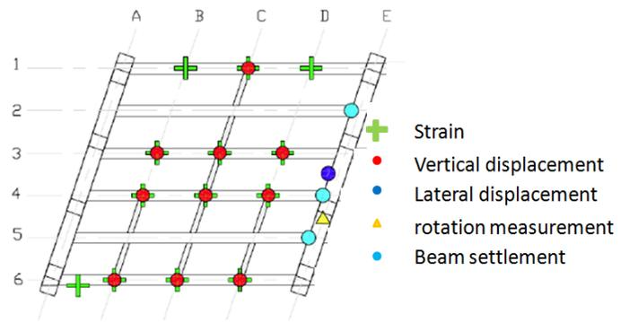
Figure 2. Static instrumentation layout for the 1<sup>st</sup> span.
