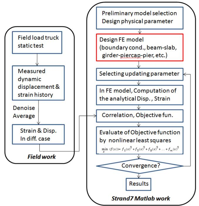
Figure 4. Flowchart of the parameter identification process based on Strand7 API function.
