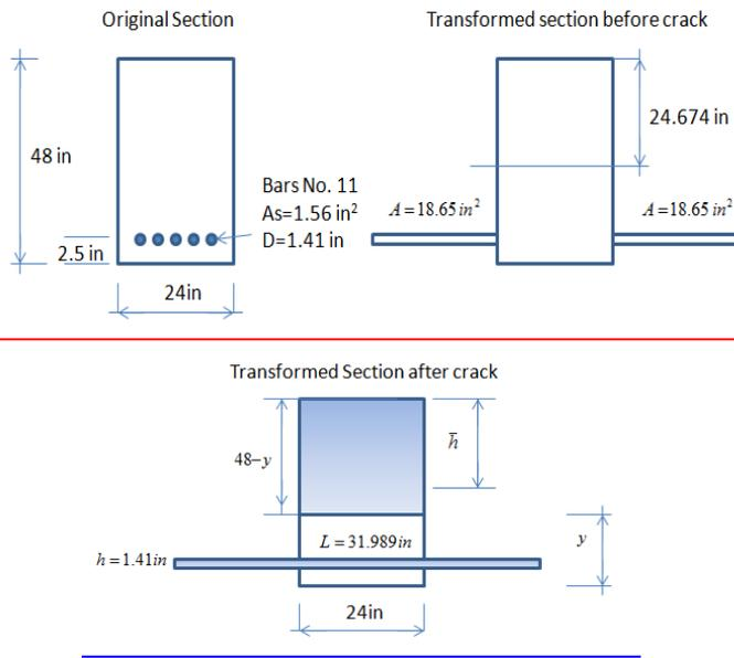
Figure 7. The girder section properties of the Smithers Bridge before and after crack appears.
