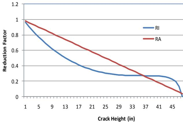
Figure 8. The relationship of RI and RA with crack height  $y$ .
