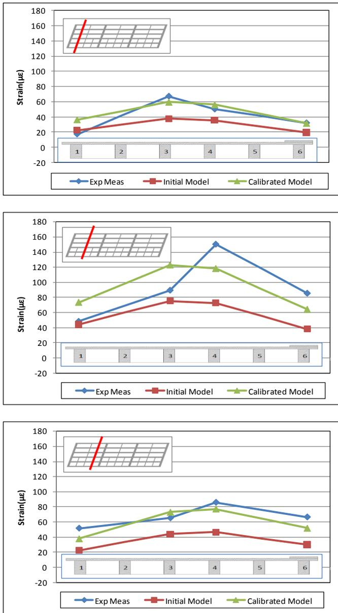
Figure 10. Comparison of strains before and after the average crack height y updating for 1/4, 1/2 and 3/4 line.
