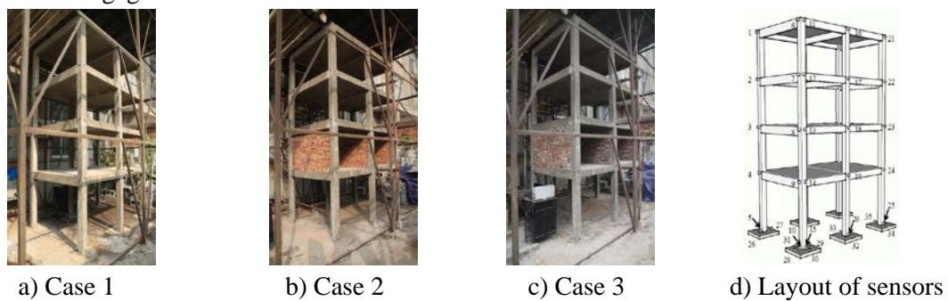
Fig. 1. Three cases of modal test and the layout of sensors
