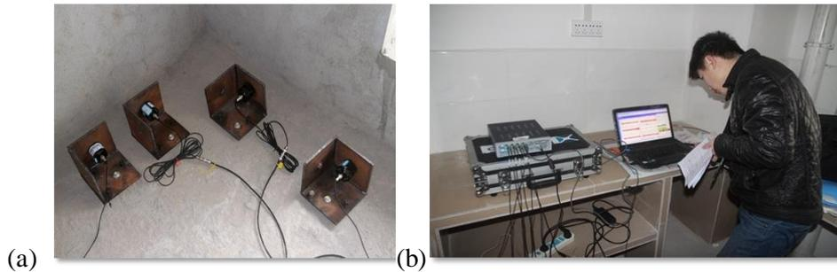
Fig.2 (a) Four accelerometers setup for one case; (b) Data acquisition test station
