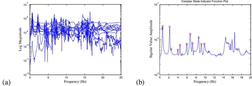
Fig.6 (a) Overlapped P-FRF; (b) Singular value of CMIF method
