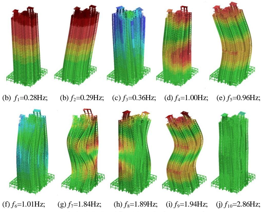
Fig.8. Calculated first 10 modes in PKPM software
