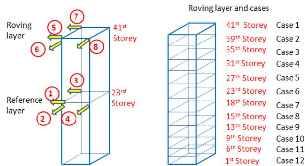
Fig.4 Roving instrumentation cases
